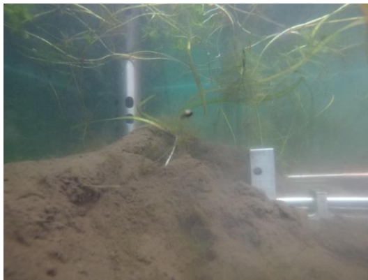
Figure 24. Substrate pile in front of tines after a trial. Trials had been performed along the width of the tank prior to the taking of this picture. The substrate mound is wider in this figure than in Figure 23.
