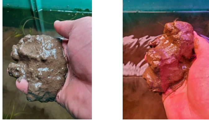
Figure 6. Muck (l) and muck/sand mix (r) substrate types were used for testing. The bulk density of muck was 36% less than the bulk density of the muck/sand mix.
