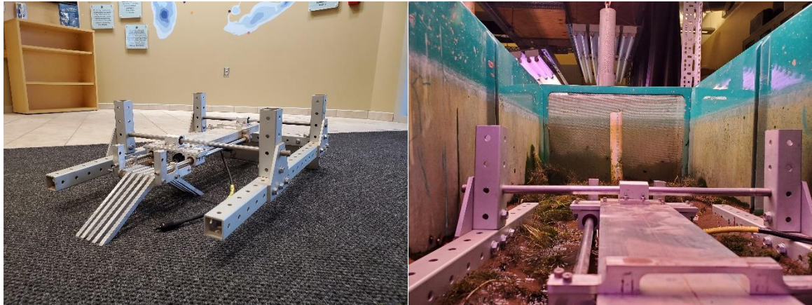
Figure 5. The tines and fin protruded below the test fixture frame (l), and the test fixture frame sat on top of the substrate (r)
