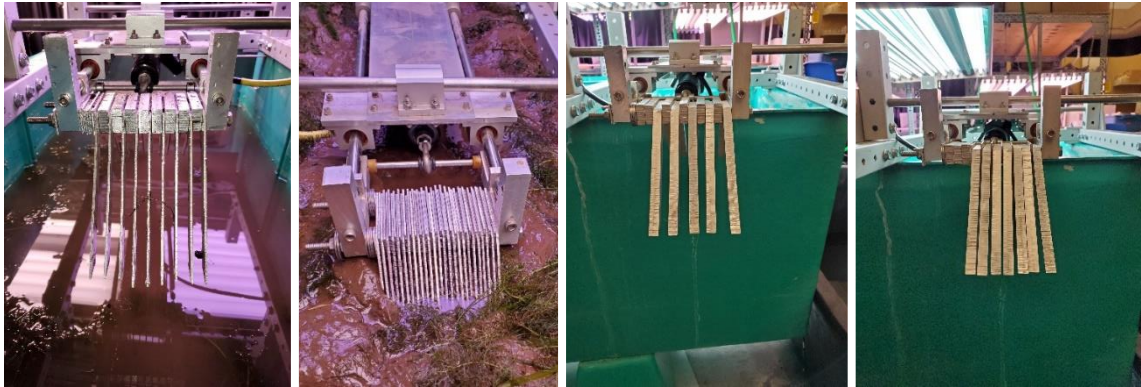
Figure 19. From left to right, nine 2.03mm tines with 9.53mm spacing, 25 2.03mm tines with 2.03mm spacing, five 9.53mm tines with 9.53mm spacing, and 9.53mm tines with 2.03mm spacing. Although the picture here contains just seven tines, the 9.53mm tines/2.03mm spacing configuration was tested with eight tines.
